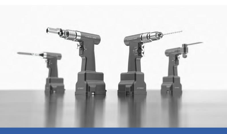
Karınca motor systems are designed in a way that all electronic components like electric circuits, brushless motor, battery cells, etc. are kept away from the sterilization. The system is divided into two parts as hand piece which is completely mechanical, goes into autoclave and power box which is completely electrical and not exposed to sterilization. This way while the service need of the system decreases, its life time increases.
